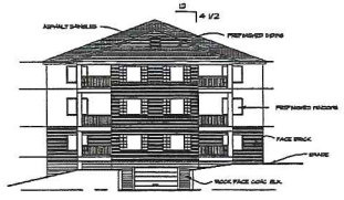
END ELEVATION SCALE 3/8" = 1'-0"
