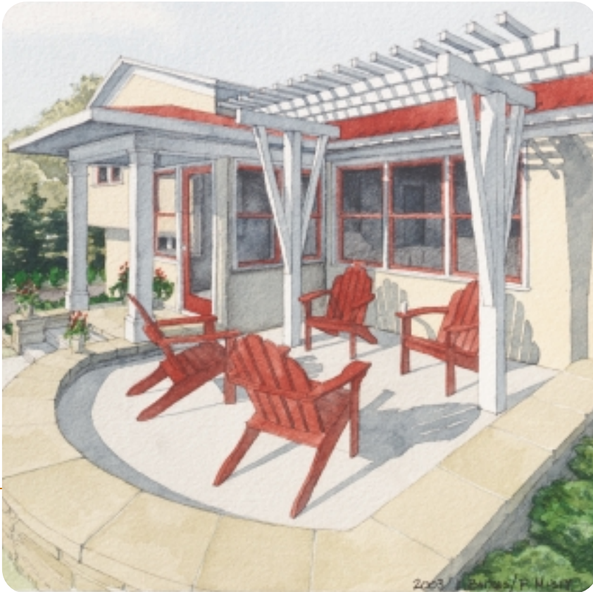
The pergola and patio recreate the pleasures of a traditional front porch. The pergola shades the patio while still allowing natural light into the living room.
