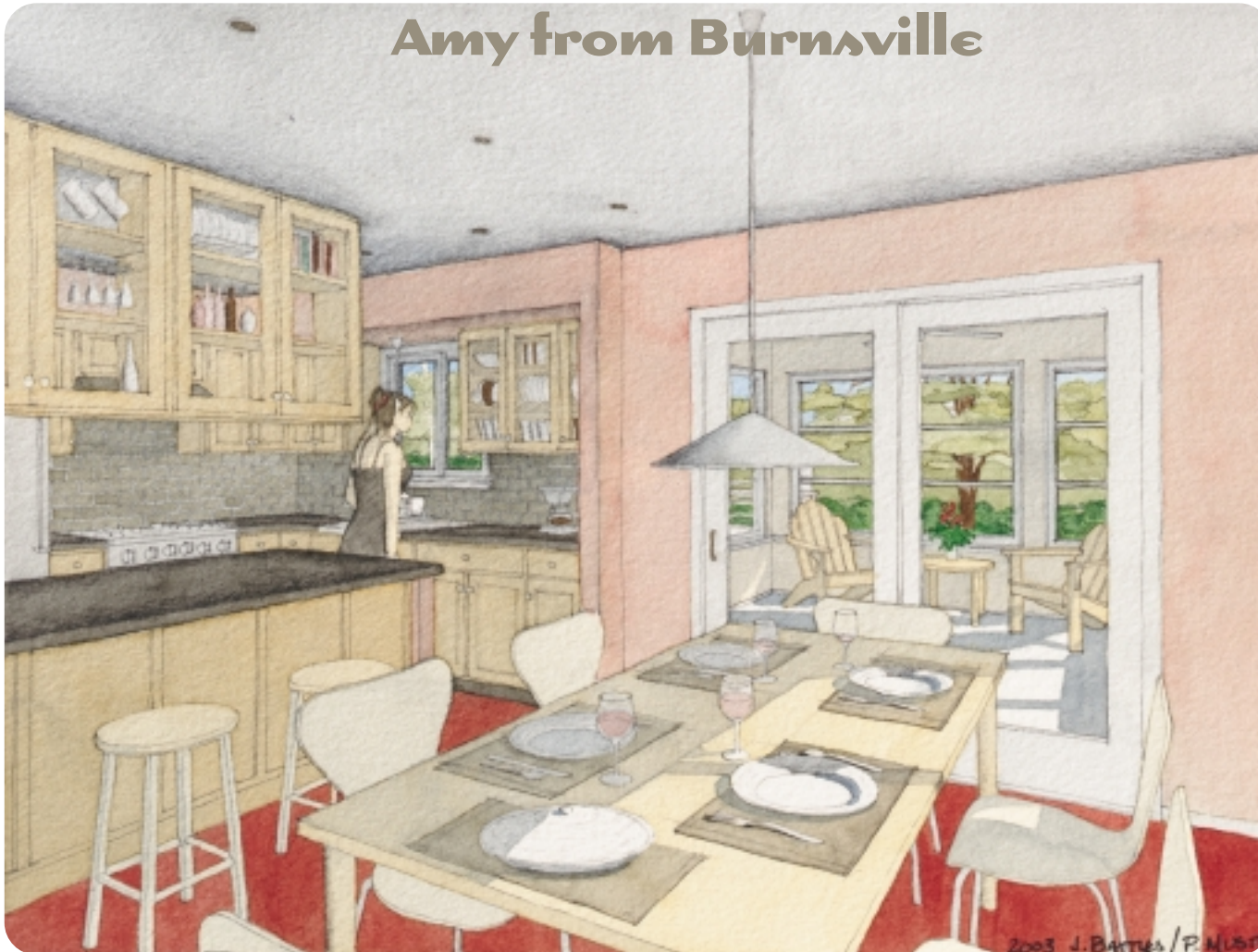
Removing part of the existing wall between the kitchen and the dining room and adding a peninsula with glass doors on the upper cabinets makes the two rooms feel larger, lighter, and more connected, while providing ample storage space. The dining room now flows onto the new four-season porch, connecting the house to the backyard.
