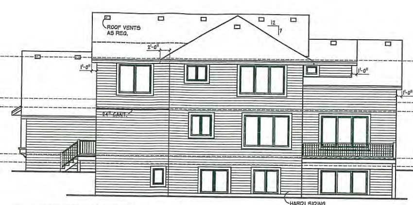
6" WINDOW & DOOR TRIM TYP. REAR ELEVATION SCALE: 1/8" = 1'-0"
